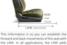
forward and back movements of the seat with the LINK. In all applications, the LINK adds power forward and backward movements, regardless of the seat's original functions. In some applications, the travel is limited. The seat adjustment information will allow you to confirm if the installation of the LINK will be suitable for your client's needs.
