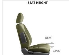
This information will give an idea of the seat height with the LINK installed. Due to the various seat styles offered by vehicle manufacturers, the information is supplied as a reference to assist you in establishing if the seated height on the LINK will be suitable for your client. *Example:* In the 2015 Ford F-150 Super Cab – the note reads as follows:
